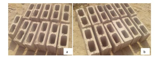
Fig. 2. a. Blocks produced from 0% sawdust replacement for sand. b. Blolocks produced from 2% sawdust replacement for sand
