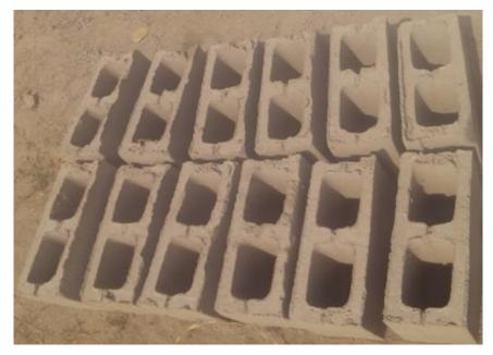
Fig. 2. Blolocks produced from 4% sawdust replacement for sand
