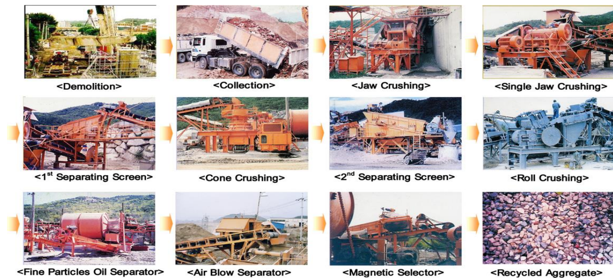
Fig 2. Recycled aggregate manufacturing process
