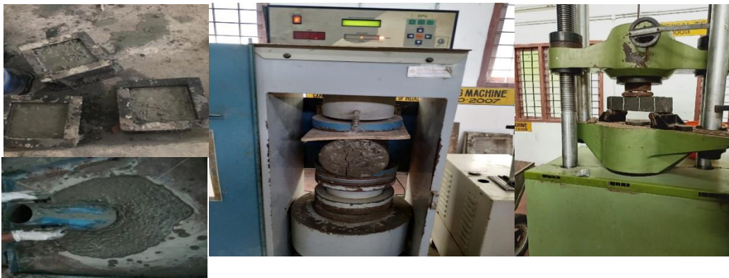
Figure 2. Slump flow test and casted specimens
